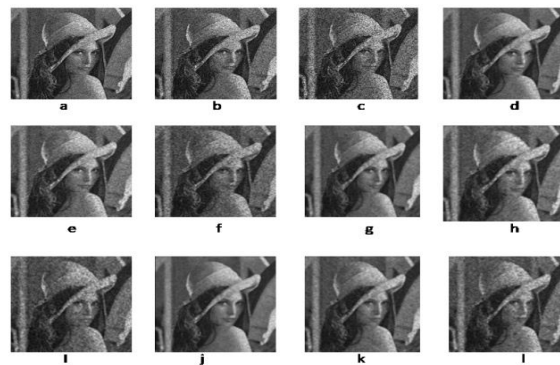
Fig.8.Noisy and restored images: Speckle noisy image with noise strength (a) SNR=10dB, (b) SNR=5dB, (c) SNR=0dB. Restored images (d) for SNR=10db using FA-NLMF, (e) for SNR=5dB using NLMF, (f) for SNR=0dB using FA-NLMF, (g) for SNR=10dB using FA-NLMF-L, (h) for SNR=5dB using FA-NLMF-L, (i) for SNR=0dB using FA-NLMF-L, (j) for SNR=10dB using FA-NLMF-C, (k) for SNR=5dB using FA-NLMF-C, (l) for SNR=0dB using FA-NLMF-C, filters.
